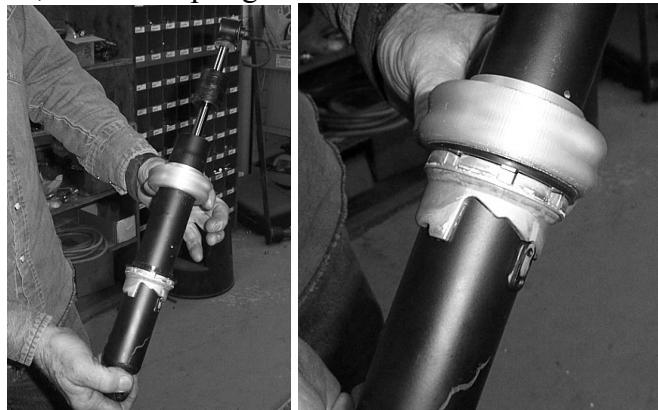
6) Place the stock spring(s) back onto the shock.
